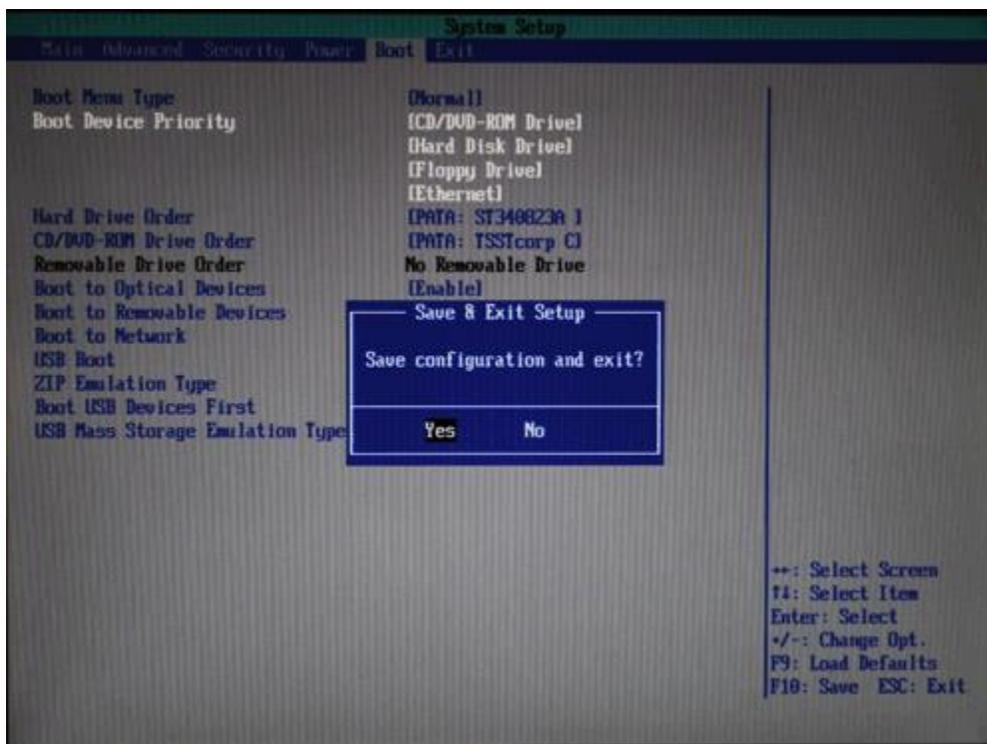
4. Make required changes in the section '**Boot Device Priority**' and press **<F10>** function key to save changes and exit BIOS settings.
