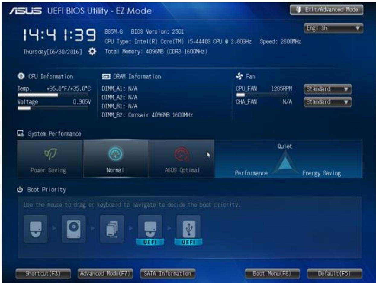
4. Click on **Advanced Mode** button or press <F7> function key to enter **Advanced Mode**. **Advanced Mode** screen is displayed as shown below:
